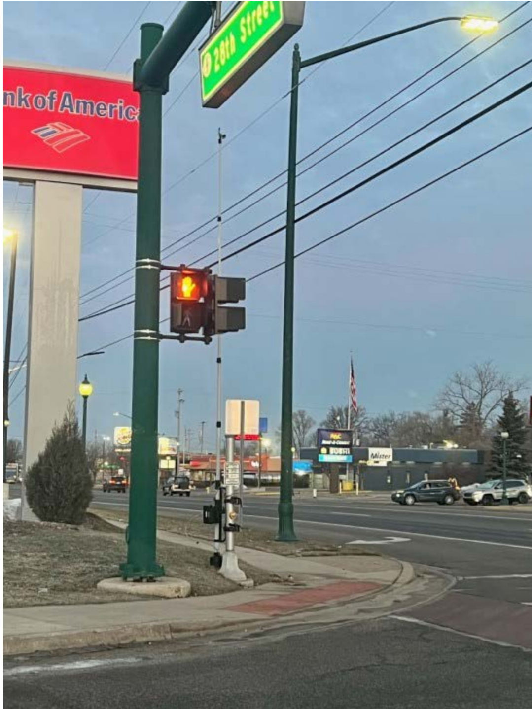
An MDOT temporary traffic counter was spotted at the intersection of 28th Street and Michael Avenue in Wyoming, Michigan. The counter is a radar camera attached to a telescopic pole and anchored to a street sign. (Courtesy Marie Bast)
