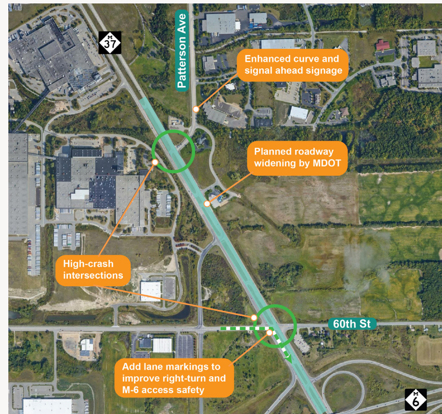
Proposed M-37/Patterson Avenue/60th Street Safety Enhancements
