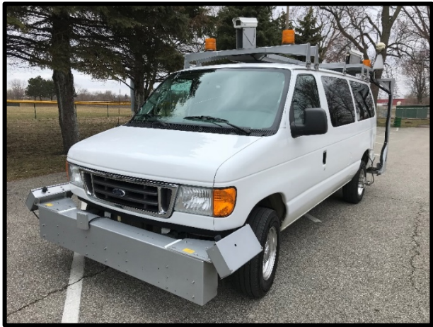
GVMC's pavement data collection van
